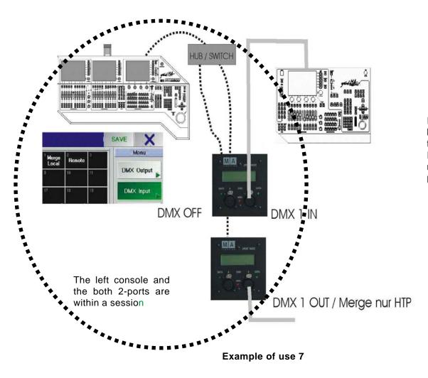
In this application example 7 – an output Universe is being controlled by the left console – the requirements for the stand-alone mode are not fulfilled, and only a restricted Merge mode is available. If on the left console, you set Universe 1 to LOCAL MERGE (in the menu TOOLS / DMX CONFIGURATION / DMX INPUT) you will only have the HTP option for the Merge mode.
