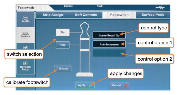
When first connecting a footswitch, touch the 'Calibrate' button to set the type of switch being used. Follow the on-screen instructions.
