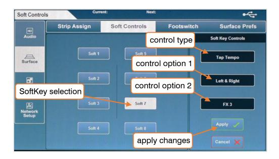
(i) When using an SQ-6, two buttons are displayed on-screen to the left of the SoftKey or SoftRotary selection buttons. Touch 'Soft Keys' or 'Soft Rotaries' to display and adjust assignments for each.
