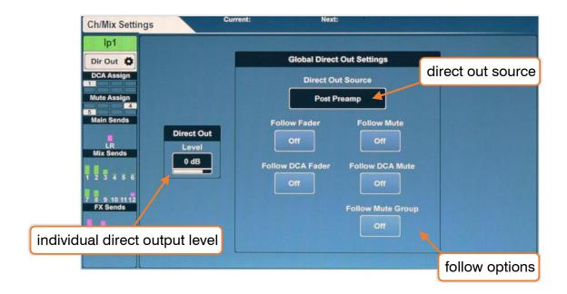
This screen shows the direct output level for the selected channel, as well as the global direct out settings which affect all channels. The currently selected channel is displayed on the left.
