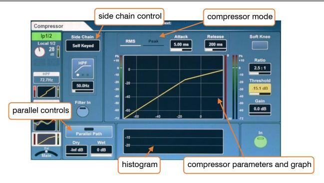
Switch the Compressor in or out using either the on-screen 'In' button or the physical Compressor 'In' key (to the left of the dedicated Compressor threshold rotary).
