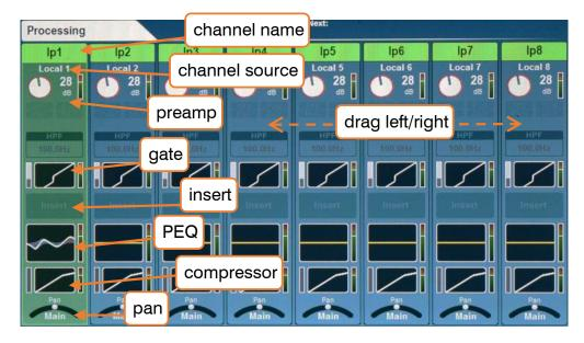
This gives the processing overview for 8 channels at once, with the selected channel highlighted. The view will automatically change if a channel is selected which is out of view, though you can also touch and drag to see all channels for the current layer. The selected mix channel is displayed to the far right.
