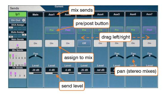
This screen displays all sends and mix assignments for the selected channel.
