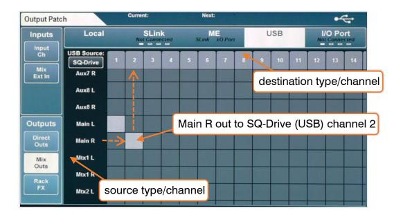
USB patching is for SQ-Drive or USB-B streaming connections. SQ-Drive uses input and output USB channels 1 to 16 and USB-B uses input and output USB channels 1 to 32.
