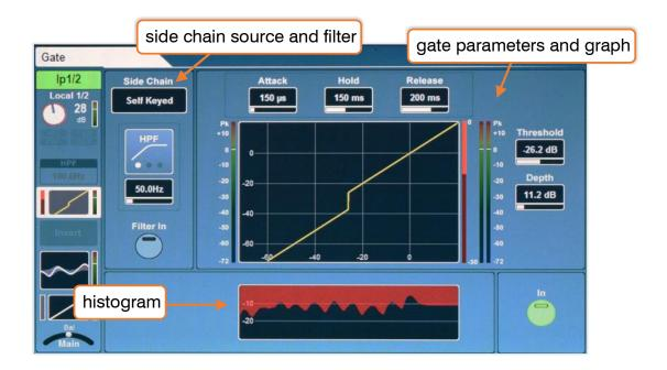
Switch the Gate in or out using either the on-screen 'In' button or the physical Gate 'In' key (to the left of the dedicated Gate threshold rotary).
