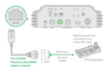
12. Or you can use CAT5/6 T-568B Standard Ethernet cable direct connect between the camera and the controller to make RS422 connection by following the pin definition below:
