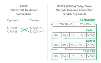
Use extension cables included RJ45 to RS422 Phoenix connecter adaptor to make RS485 connection for your control device.
