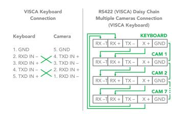
Use extension cables RJ45 to RS422 Phoenix connecter adaptor included to make RS422 connection for your control device.
