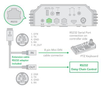
10. Use extension cables included RJ45 to RS422/232 Phoenix terminal contact adaptor to make RS232 connection for your control device.
