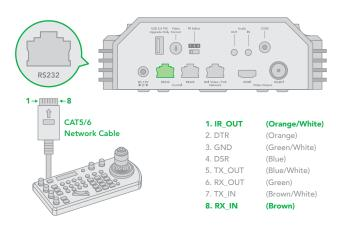
12. How to make RS232 Daisy Chain multiple camera connection with standard RS232 serial port controller as below:
