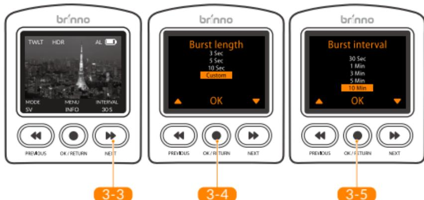
**!** 30 Sec Burst Interval option is only for **3 Sec** Burst Length mode.
