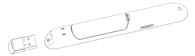
3) Plug the USB receiver into the USB port.
